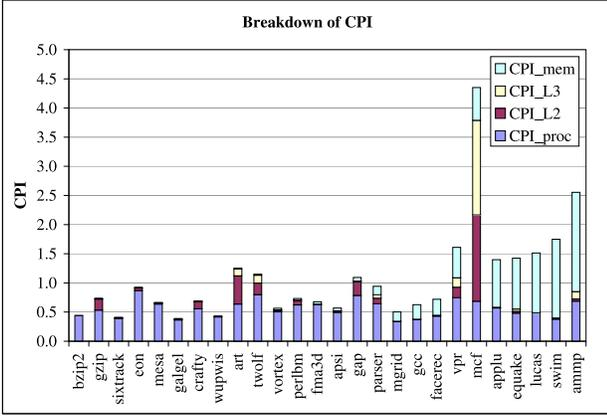
Figure 1: CPI breakdown of SPEC2000 applications. The applications are sorted by the increasing order of their  $CPI_{mem}$  values.  $CPI_{proc}$  corresponds to the cycles spending on the processor execution and L1 cache accesses; while  $CPI_{L2}$ ,  $CPI_{L3}$ , and  $CPI_{mem}$  correspond to the cycles due to accesses to the L2 cache, L3 cache, and main memory, respectively.
