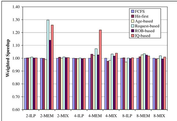
Figure 10: Performance comparisons of thread-aware scheduling schemes (Request-based, ROB-based, and IQ-based) with the schemes that treat accesses from different threads the same (FCFS, Hit-first, and Age-based).
