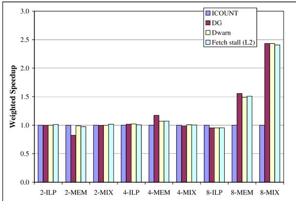
Figure 2: Performance comparisons of four fetch policies on an SMT system with the 2-channel DDR SDRAM system.
